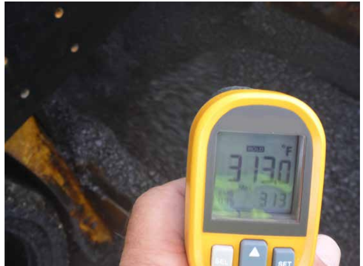
Plant Production Temperature – Increase and maintain at high end of acceptable production range.
